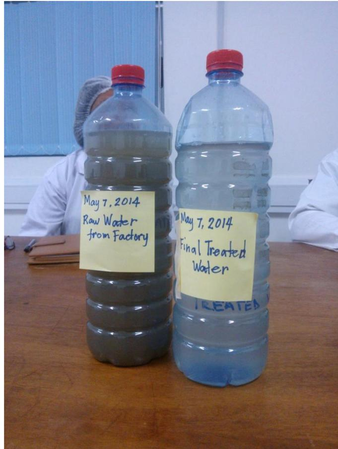
**Fig 6. Comparison of Raw Water & Treated Water Samples**
